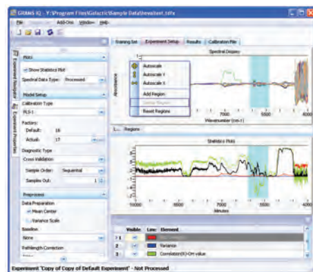
The Experiment Setup tab region selector offers correlation tools to guide selection of the best spectral regions for calibration.
